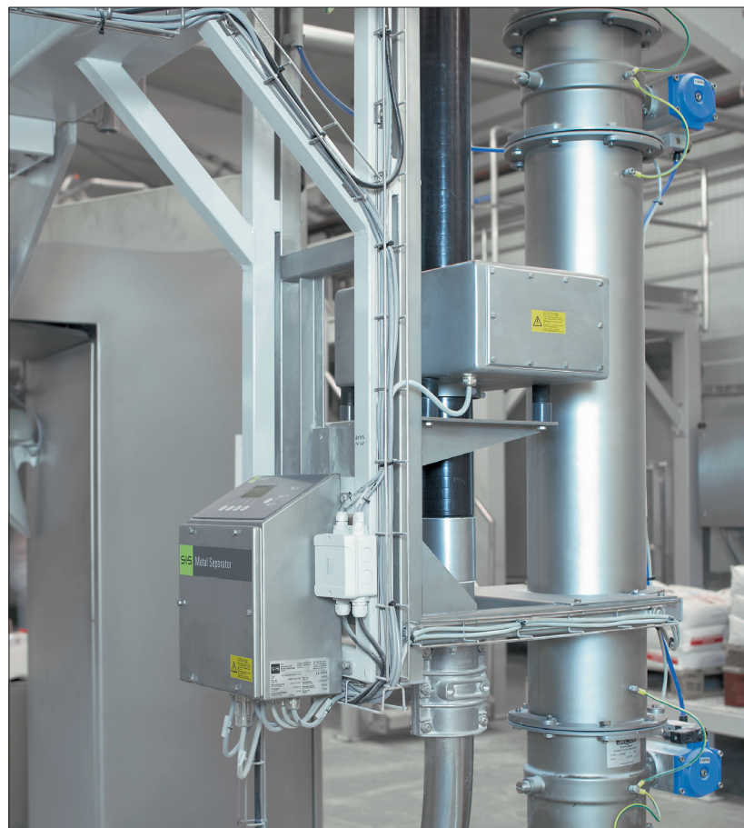
Sesotec GF 4000 integrated into a pneumatic conveying line.
